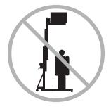
Do not raise unless the load is properly secured to the forks.
