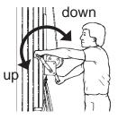
4 Lower the load by firmly grasping the winch handles and rotating them away from the mast. After lowering to the desired position, turn the winch handles toward the mast (raise the load) <sup>1</sup>/4 turn to set the brakes.
