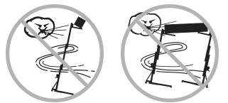
Do not leave a load raised when windy conditions may occur unless the machine(s) are properly guy-wired.
